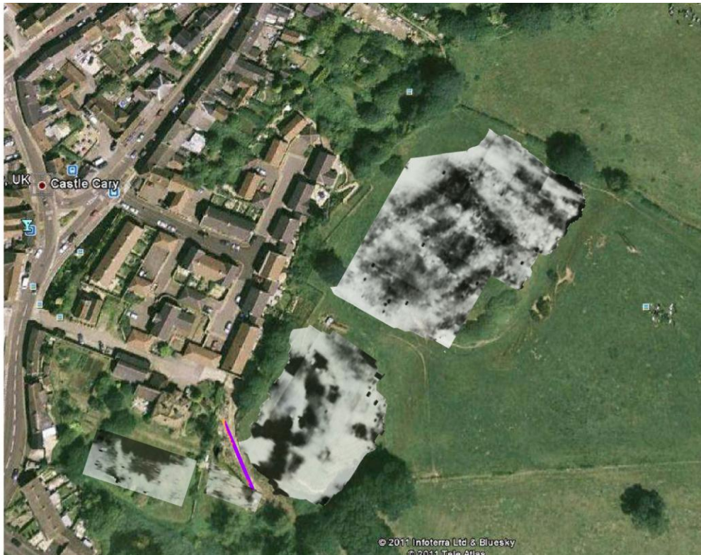
Figure 4.2 Showing both the resistance survey and second radar survey at Manor Farm with the resistance survey at the castle site.
