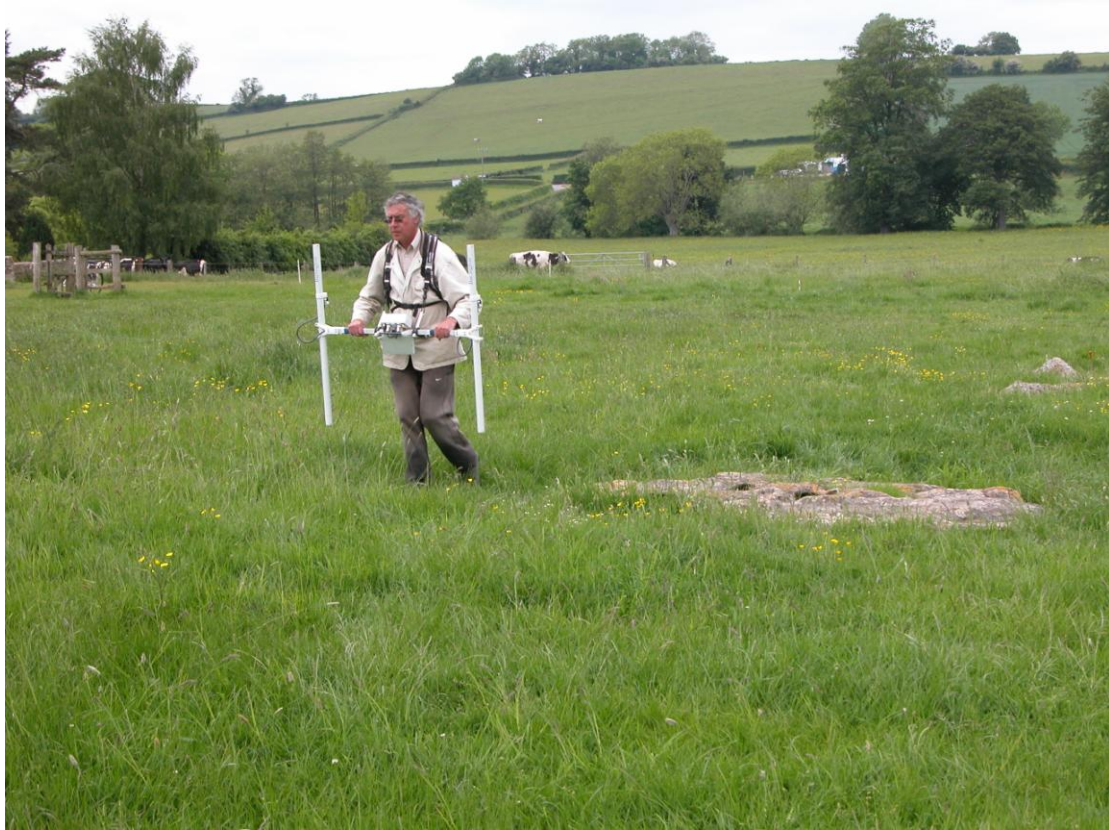
Figure 2.1. Bartington 601-2 twin fluxgate gradiometer
