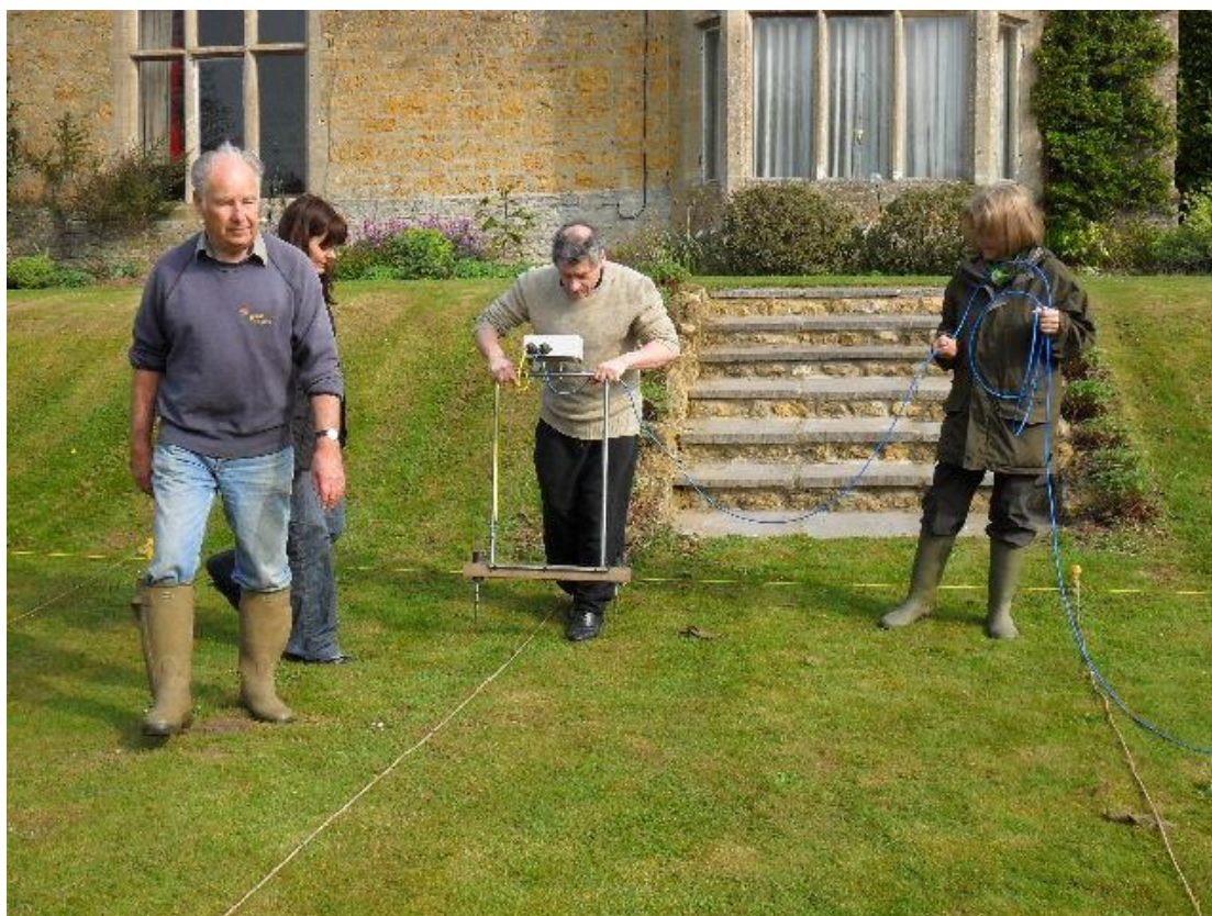
Figure 2.2 The TR/CIA twin-probe resistance meter
