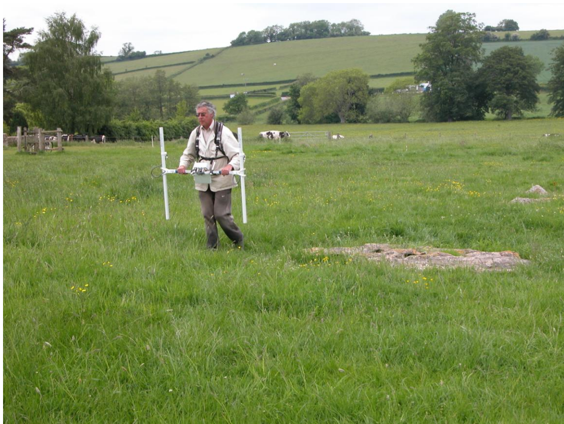
Figure 2.1 Bartington 601-2 twin fluxgate gradiometer.
