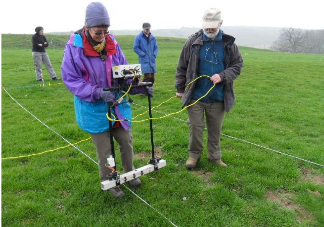
Figure 2.2 twin-probe resistance meter
