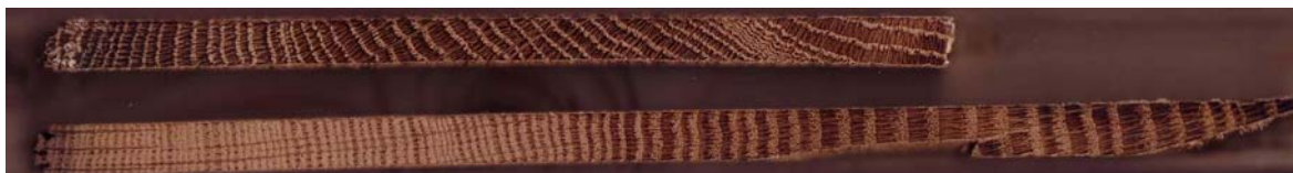
Photo 4: An example of the tree-ring series revealed through the sanding of cores
